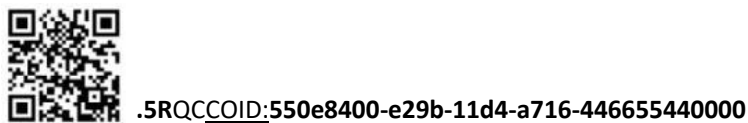
Figure 15 UUID code with responsibility provided by DI “5R”, IAC “QC” and Company ID “COID”.
